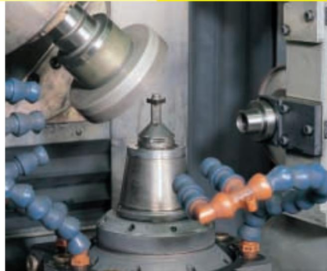
**These grinding machines were converted by our 'jig construction' department according to our concepts**
