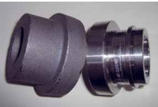
Forged Blank and ready machined workpiece
