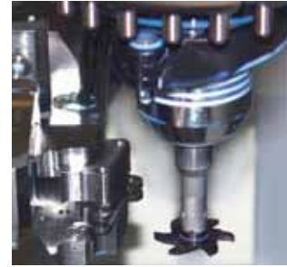
Picture, top: The slots are milled in the two jaw sections with the slot miller 636.
