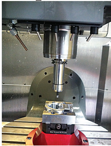
A cutting tool clamped in a FAHRION CENTRO/P precision collet chuck machines a part during a Haas machine tool demonstration.
