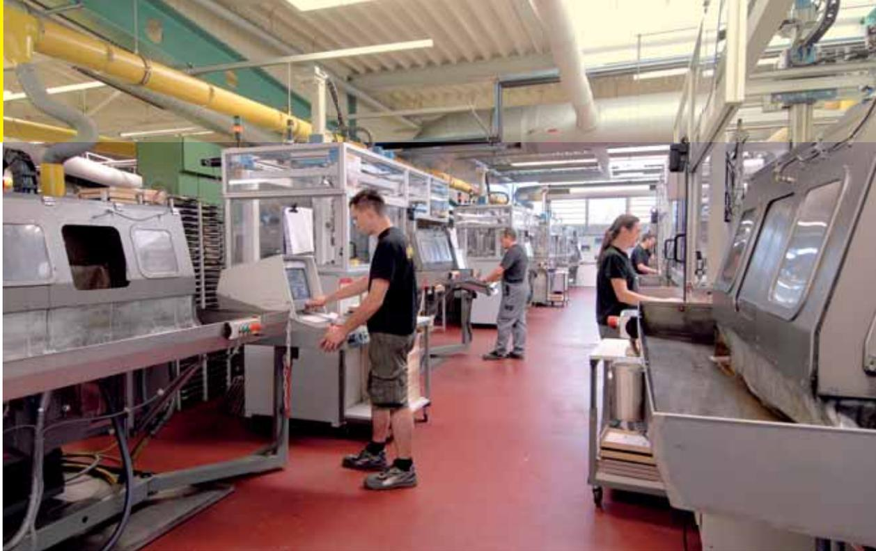
View into the grinding section for inserts of the Supermini® range
