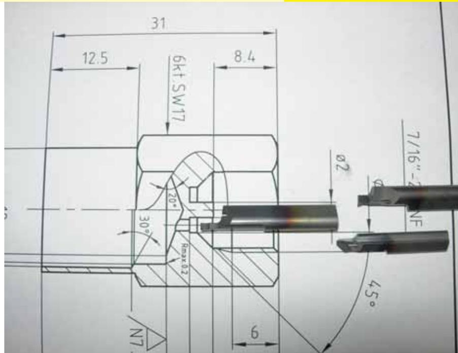
The positioning of the Supermini® inserts relate to the contours of the pressure sensor housing which are to be machined
