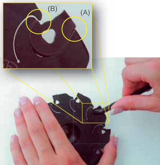
The location and fixation of the insert in the cutter body is quite simple
