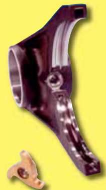
Milling a groove in the shift fork with an insert type 328 is the next project.
