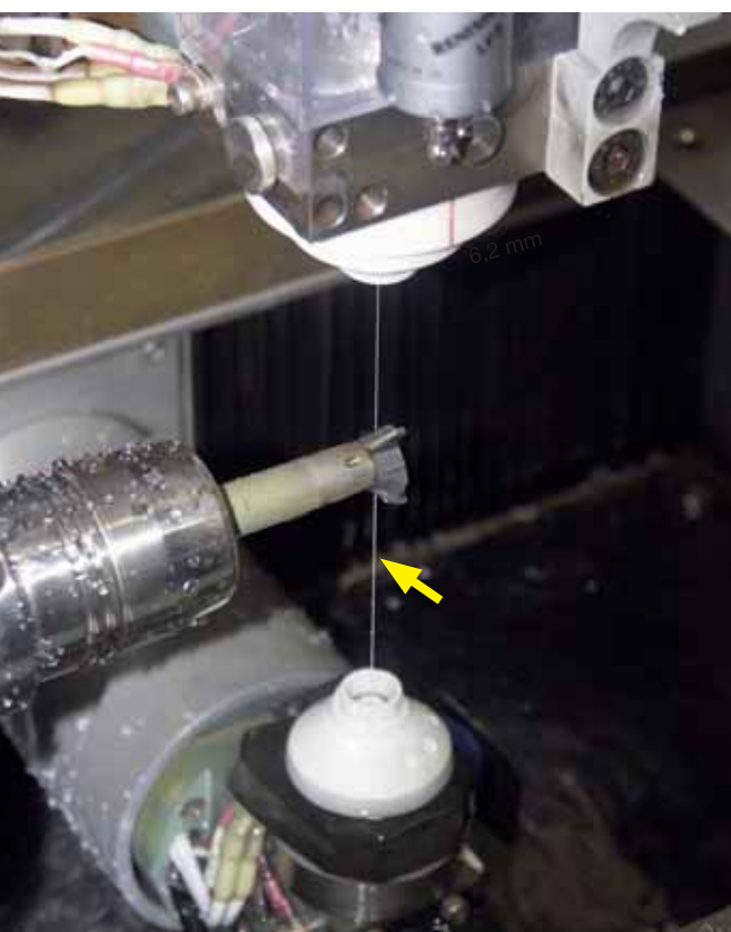
Erosion of a CBN special insert. The diameter of the wire is 0,03 mm
