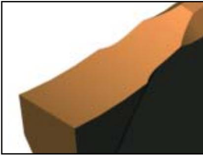
Figure 1: A simple radial-ground top rake geometry.
