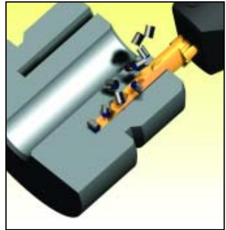
Figure 4: With face grooving, chip control is difficult because the chip is not flowing directly into the insert geometry, but, instead, is moving across it.
