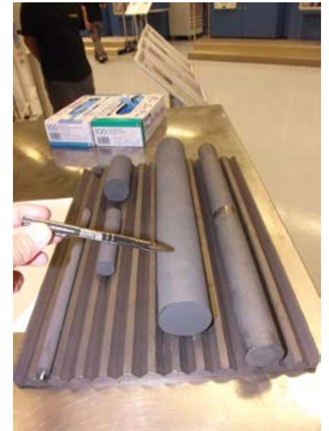
The semi-finished preforms ready for downstream shaping and sintering. Sintering is perhaps the most important part of the insert-making process, and methods are a closely guarded secret. Photography was prohibited in the sintering department, but the equipment was seen to have very large capacity and computer control.
