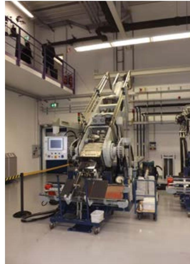
Raw materials for inserts that start life as a powder must be pressed and sintered into a final shape. This machine extrudes the powder into stick-like preforms for further processing
