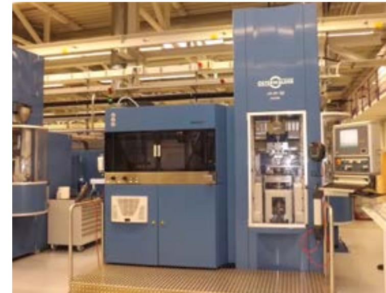
This machine uses a process called isostatic pressing to compress the powder into shape with the same force over the whole surface area of the insert. Complex shapes that can't be molded using conventional equipment can be processed.
