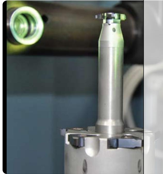
such as Wayne Ballenger indexed the inserts and measured them on a presetter to ensure proper insert positioning.
