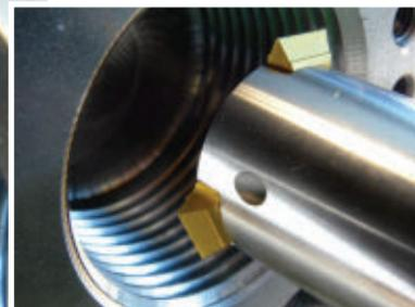
to moving over to thread milling. “Programming a thread mill is a three axis move. With some of them, you have to understand how to arc into the cut correctly,” says John Kollenbroich, technical manager, Horn USA Inc., Franklin, TN.
