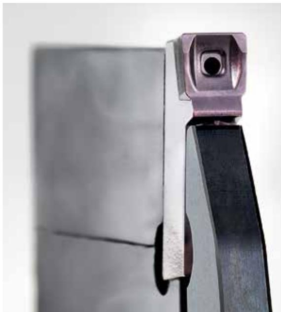
Horn says its new S100 insert for grooving and parting-off precisely delivers lubricating and cooling fluids. The “.3V” chipbreaker geometry and wear-resistant TiAlN coating for machining stainless steels is an expansion of the existing S100 system. The coolant port works directly at the cutting zone and creates a focused coolant jet, reducing the chance of built-up edge and assisting in chip formation.
