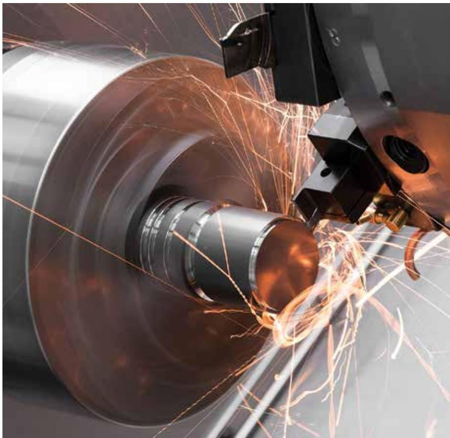
Hard turning with PCBN tools is possible under dry conditions.
