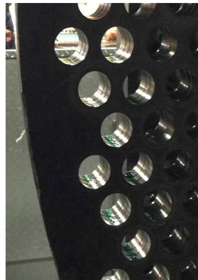
Milling the two tiny grooves inside each bore consumed 25 percent of the part's total cycle time when using a 3-flute cutter, Cambron's original approach.
