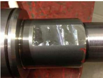
According to Kischnick, “The challenge was to mill a 1.500” long flat, .060” deep on a shaft using a .854” diameter cutter hanging more than 10” out of the spindle. Not an easy task, but one I felt we could accomplish with the right tool.
