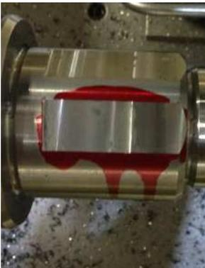
The cutter MT&G was attempting to use was a staggered flute design that caused pushing and pulling during the cut. After careful analysis it was clear that we should try a Mini Mill insert from Horn USA that would apply all cutting forces downward and free up the cut, utilizing a positive axial helix.”
